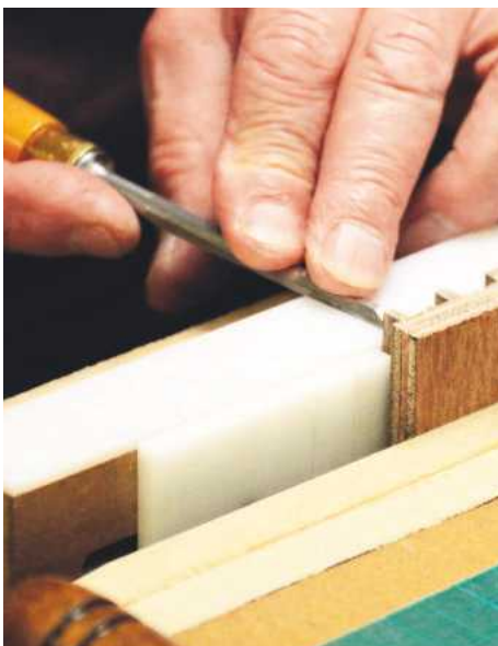
After sawing, the second jig is used to pare the base of the pins flat and square
